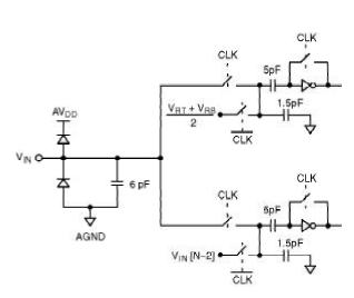
Figure 4. Equivalent Input Circuit
