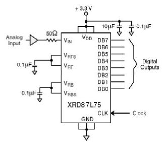
Figure 5. Typical Circuit Connections
