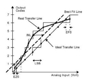
Figure 3. INL Error Calculation
