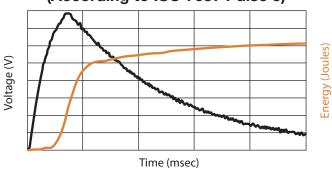
When using the test method indicated below, the amount of Energy dissipated by the varistor must not exceed the Load Dump Energy value specified in the product table.
