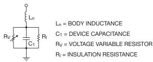
Figure 4. Antenna Varistor
