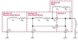
Where:  $C_H$  = Lumped capacitance between the human body and earth
