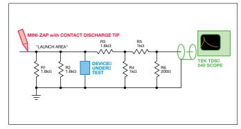
Figure 2. Schematic of Test Set Up
