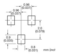
Figure 1B. SOT23- Solder Pad Layout
