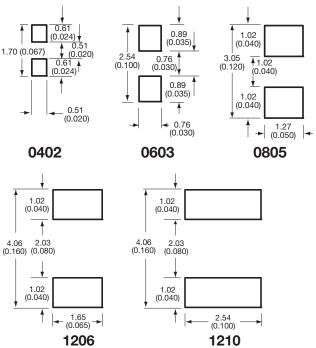
Figure 1: TransGuard® Solder Pad Dimensions
