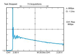
Figure 3. Open Circuit Response of Test Fixture to an Injected ESD Waveform
