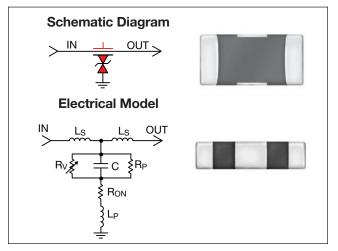
inductance, is the enhanced attenuation characteristics of the TransFeed product. Not only is there significantly greater attenuation at a higher self-resonance frequency, but the roll-off characteristic becomes much flatter, resulting in EMI filtering over a much broader frequency spectrum. Typical applications include filtering/protection on Microcontroller I/O Lines, Interface I/O Lines, Power Line Conditioning and Power Regulation.
