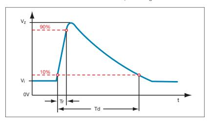
When using the test method indicated below, the amount of Energy dissipated by the varistor must not exceed the Load Dump Energy value specified in the product table.
