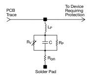
Where:  $R_V$  = Voltage Variable resistance (per VI curve)
