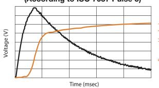
When using the test method indicated below, the amount of Energy dissipated by the varistor must not exceed the Load Dump Energy value specified in the product table.
