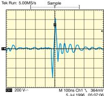
connected to the scope and one leg of the relay/motor coil; the probe's ground was connected to the other relay coil/motor wire. The scope was triggered on the pulse and waveforms printed.
