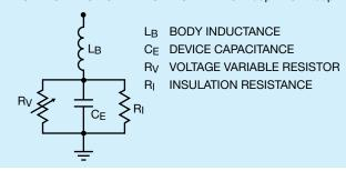
Figure 2. TransGuard® Equivalent Model.
