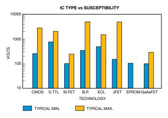
Figure 3. IC Type E Field Susceptibility
