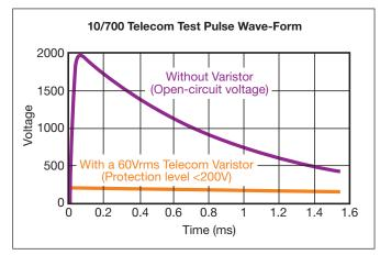
Ten pulses with a duration of 10x700µs applied at one minute intervals are specified for telecom equipment.
