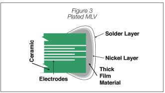
In the plated termination, the base termination layer is still used (it provides contact from the electrodes to the circuitry). On top of the base termination is a layer of nickel. This is the surface to which the solder bonds during assembly. It must be thick enough to stay intact during IR reflow or wave
