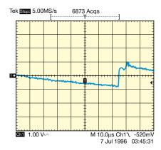
Fig. 6. 12 V Relay Transient without protection 105 V 50 V/Division
