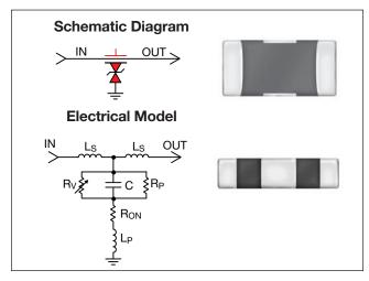
the TransFeed product. Not only is there significantly greater attenuation at a higher self-resonance frequency, but the roll-off characteristic becomes much flatter, resulting in EMI filtering over a much broader frequency spectrum. Typical applications include filtering/protection on Microcontroller I/O Lines, Interface I/O Lines, Power Line Conditioning and Power Regulation.
