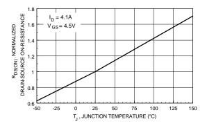
Figure 3. On-Resistance Variation with Temperature.
