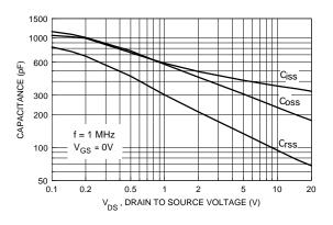
Figure 9. Capacitance Characteristics.
