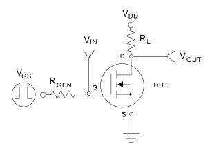
Figure 11. Switching Test Circuit.
