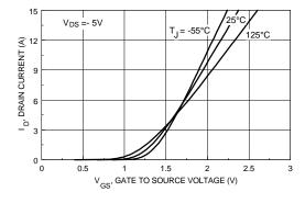
Figure 5. Transfer Characteristics.
