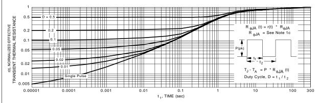
Figure 17. Transient Thermal Response Curve.
