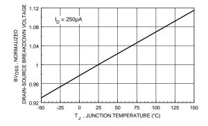
Figure 7. Breakdown Voltage Variation with Temperature.
