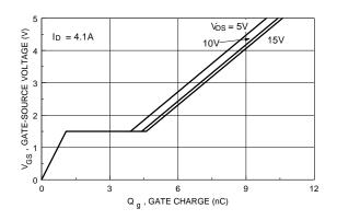
Figure 10. Gate Charge Characteristics.
