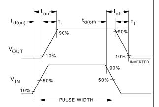
Figure 12. Switching Waveforms.
