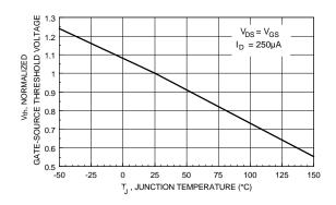
Figure 6. Gate Threshold Variation with Temperature.
