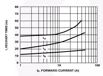
FIGURE 3. 5. TYPICAL t<sub>RR</sub>, t<sub>A</sub> AND t<sub>B</sub> CURVES vs FORWARD CURRENT
