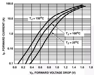
FIGURE 1. FORWARD VOLTAGE vs FORWARD CURRENT CHARACTERISTIC
