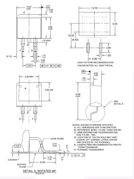
Figure 9. TO-263 2L (D2-PAK) - 2LD, TO263, SURFACE MOUNT
