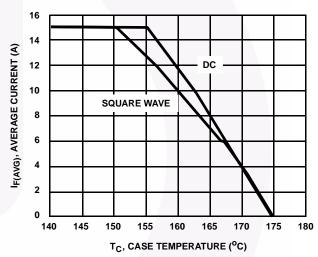
FIGURE 4. 6. TYPICAL CURRENT DERATING CURVE vs CASE TEMPERATURE
