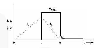
FIGURE 8. AVALANCHE CURRENT AND VOLTAGE WAVEFORMS
