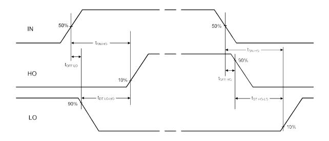
Deadtime  $t_{DT LO-HO} = t_{ON HO} - t_{OFF LO}$  $t_{DT HO-LO} = t_{ON LO} - t_{OFF HO}$
