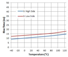
Figure 9. Rise Time vs. Temperature
