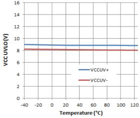
Figure 26. VCC UVLO vs. Temperature
