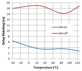
Figure 15. Delay Matching vs. Temperature
