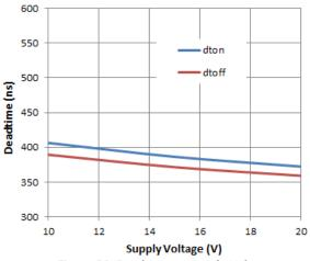
Figure 24. Deadtime vs. Supply Voltage
