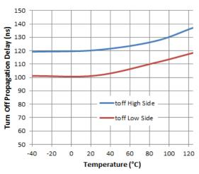
Figure 7. Turn-off Propagation Delay vs. Temperature
