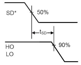
Figure 1. Input / Output Timing Diagram
