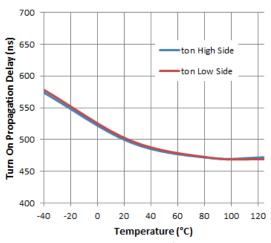
Figure 5. Turn-on Propagation Delay vs. Temperature
