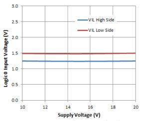
Figure 22. Logic O Input Voltage vs. Supply Voltage
