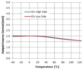
Figure 17. Output Source Current vs. Temperature
