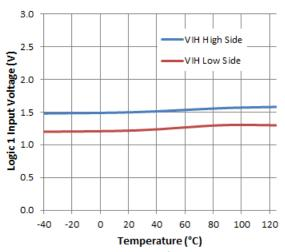
Figure 21. Logic 1 Input Voltage vs. Temperature
