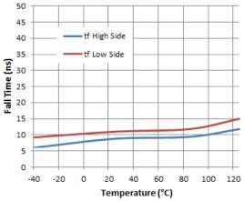
Figure 11. Fall Time vs. Temperature
