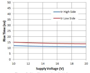
Figure 8. Rise Time vs. Supply Voltage
