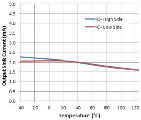
Figure 19. Output Sink Current vs. Temperature
