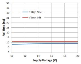
Figure 10. Fall Time vs. Supply Voltage
