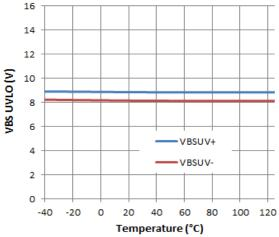
Figure 27. VBS UVLO vs. Temperature
