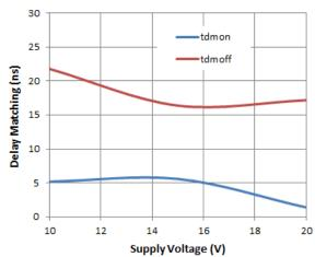
Figure 14. Delay Matching vs. Supply Voltage
