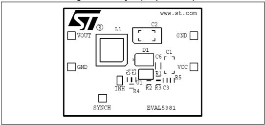
Figure 20. PCB layout (bottom side)
