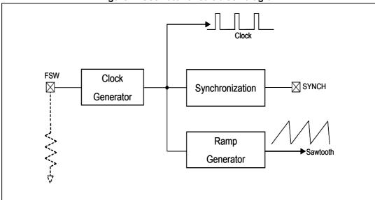
Figure 4. Oscillator circuit block diagram
