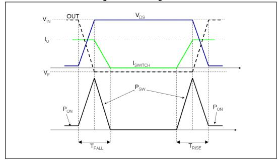
Figure 16. Switching losses
