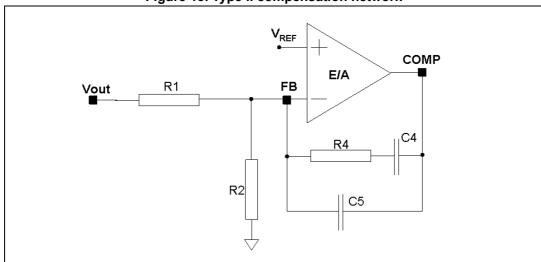
Figure 13. Type II compensation network
