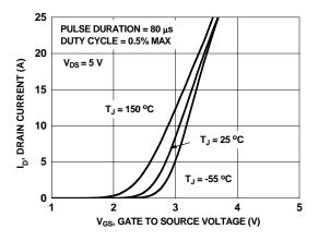
Figure 5. Transfer Characteristics
