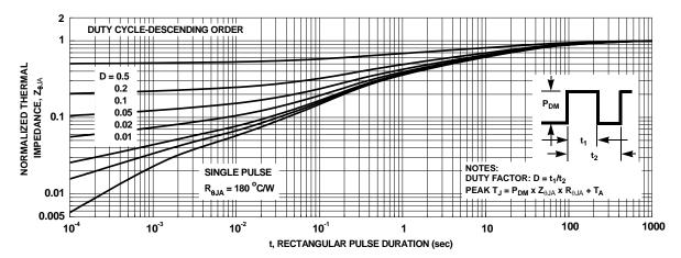
Figure 11. Junction-to-Ambient Transient Thermal Response Curve Figure 12.
