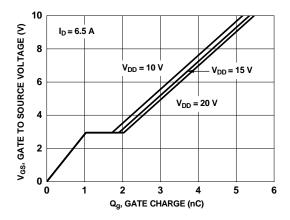
Figure 7. Gate Charge Characteristics
