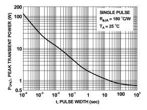
Figure 10. Single Pulse Maximum Power Dissipation
