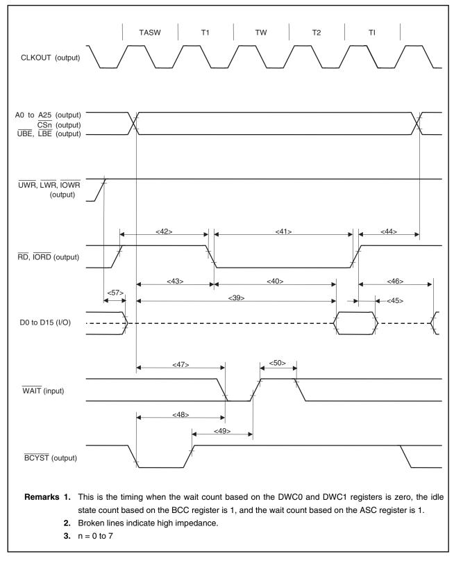
(b) Read timing (SRAM, external ROM, external I/O) (2/2)
