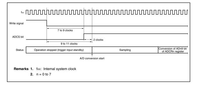
Figure 12-19. Timer Trigger Mode A/D Conversion Time (When ADM1 = 20H or 30H)
