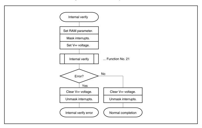
Figure 16-10. Internal Verify Flow
