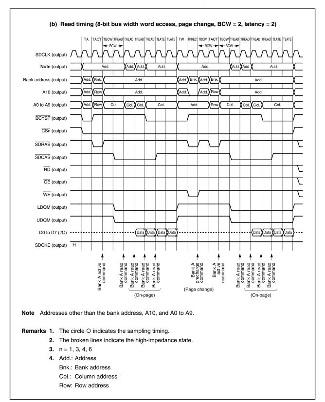
Figure 5-22. SDRAM Access Timing (2/4)
