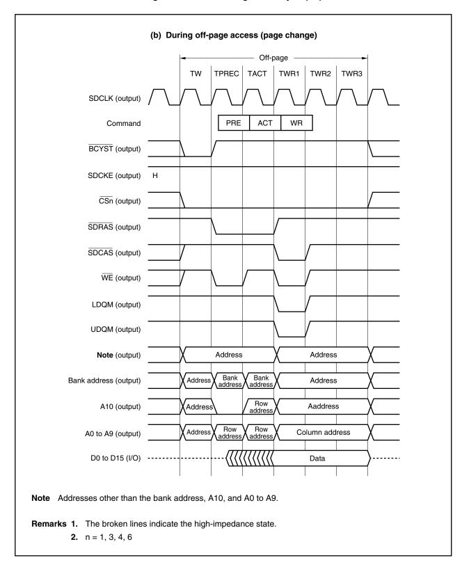
Figure 5-21. SDRAM Single Write Cycle (2/3)
