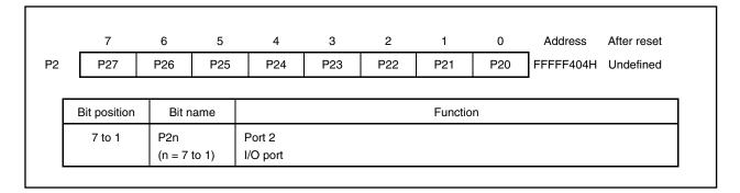
In addition to their function as port pins, the port 2 pins can also operate as the timer/counter I/O, external interrupt request inputs, and the DMA end (terminal count) signal outputs in the control mode.
