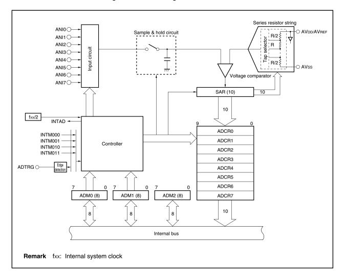
Figure 12-1. Block Diagram of A/D Converter
