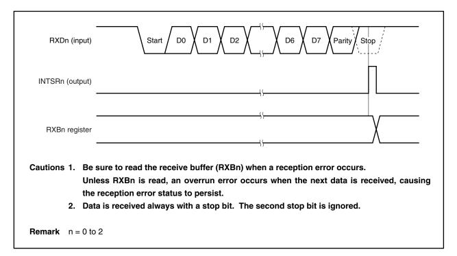
Figure 11-7. Asynchronous Serial Interface Reception Completion Interrupt Timing
