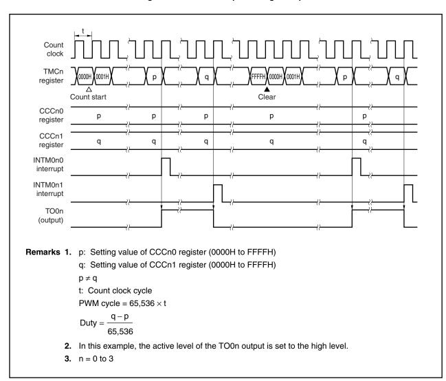
Figure 10-10. PWM Output Timing Example
