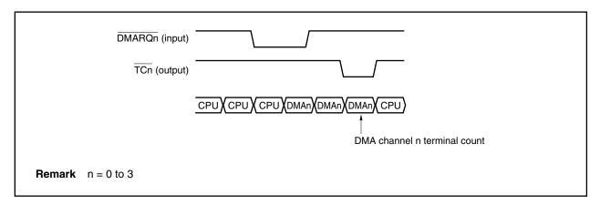
The TCn signal becomes active for one clock at the beginning of the write cycle of the last DMA transfer when 2-cycle transfer is executed.
