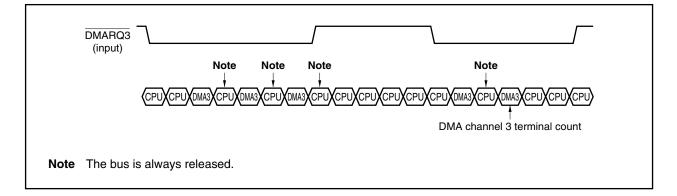
Figure 6-3 shows an example of a single transfer in which a higher priority DMA request is issued. DMA channels 0 to 2 are in the block transfer mode and channel 3 is in the single transfer mode.
