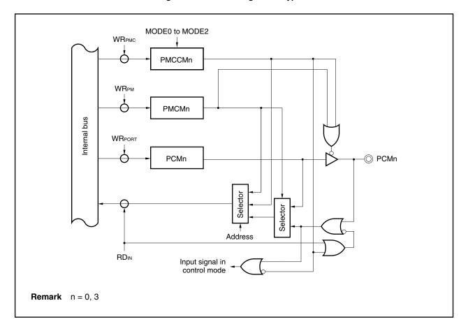
Figure 14-4. Block Diagram of Type D
