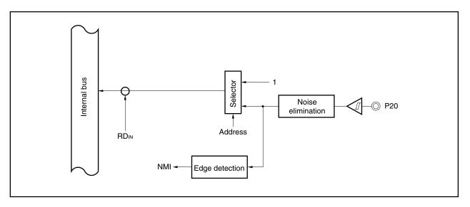
Figure 14-7. Block Diagram of Type G
