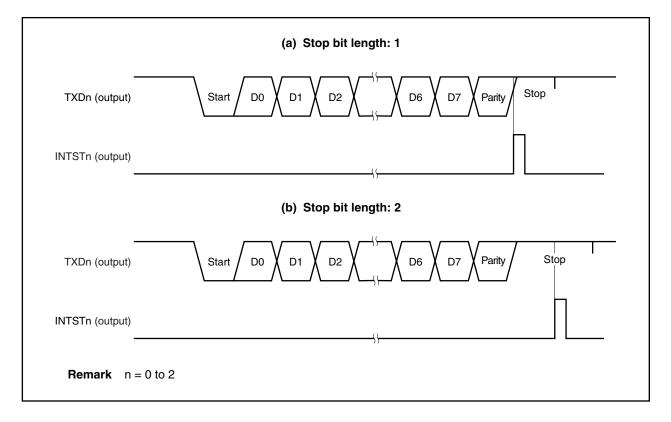
Figure 11-3. Asynchronous Serial Interface Transmission Completion Interrupt Timing
