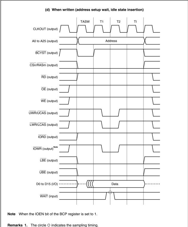
Figure 5-2. SRAM, External ROM, External I/O Access Timing (4/6)
