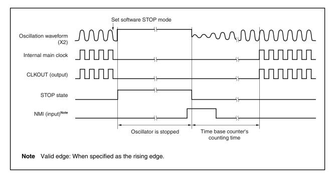
The NMI pin should usually be set to an inactive level (for example, high level when the valid edge is specified as the falling edge) in advance.
