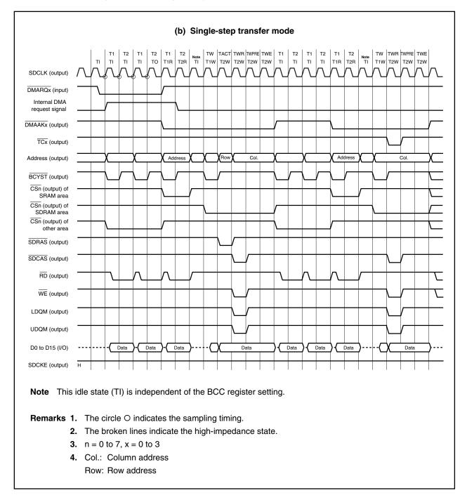
Figure 6-13. Timing of 2-Cycle DMA Transfer (SRAM  $\rightarrow$  SDRAM) (2/3)
