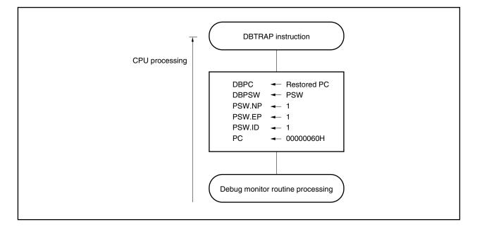
Figure 7-12. Debug Trap Processing
