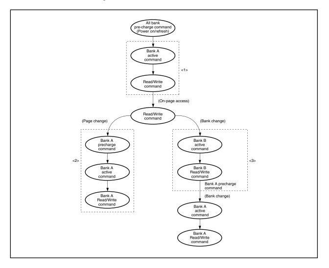
Figure 5-19. State Transition of SDRAM Access
