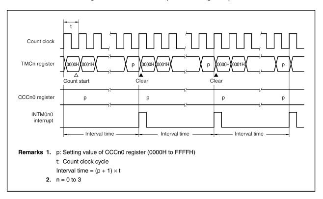
Figure 10-8. Interval Timer Operation Timing Example
