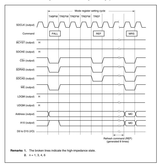
Figure 5-26. SDRAM Mode Register Setting Cycle
