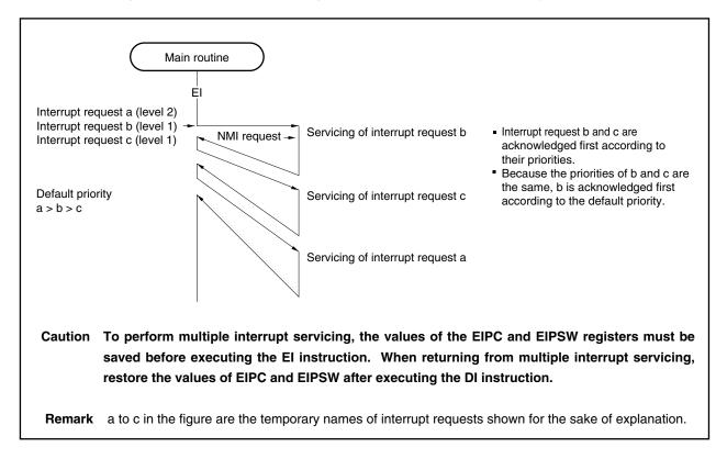
Figure 7-7. Example of Servicing Interrupt Requests Simultaneously Generated
