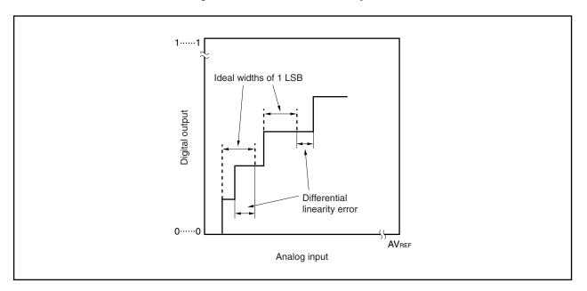
Figure 12-26. Differential Linearity Error
