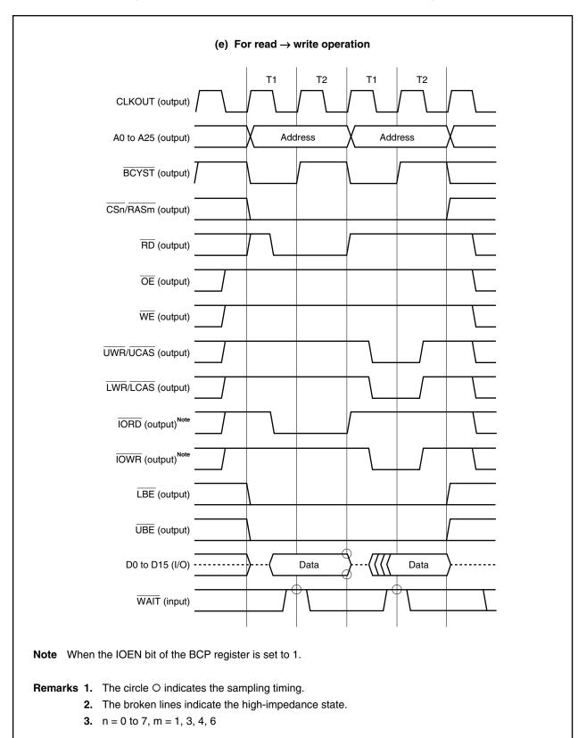
Figure 5-2. SRAM, External ROM, External I/O Access Timing (5/6)
