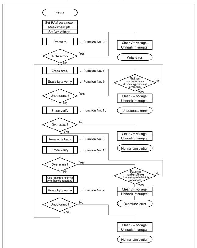
Figure 16-8. Erasing Flash Memory Flow
