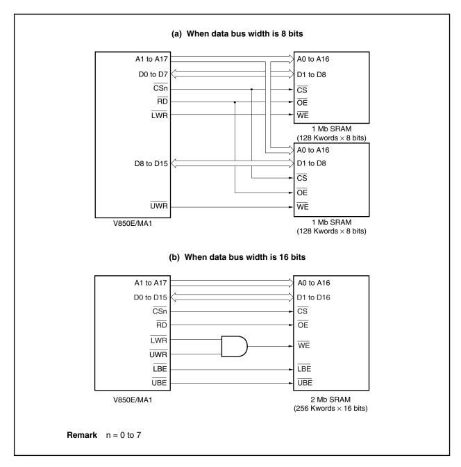
Figure 5-1. Examples of Connection to SRAM (1/2)
