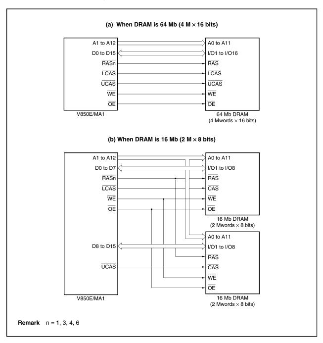
Figure 5-6. Examples of Connection to DRAM
