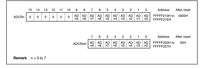
The correspondence between each analog input pin and the ADCRn register (except the 4-buffer mode) is shown below.
