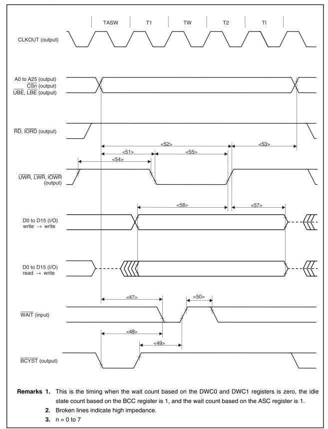
(c) Write timing (SRAM, external ROM, external I/O) (2/2)
