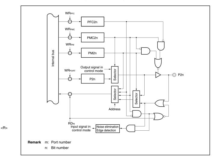
Figure 14-14. Block Diagram of Type N
