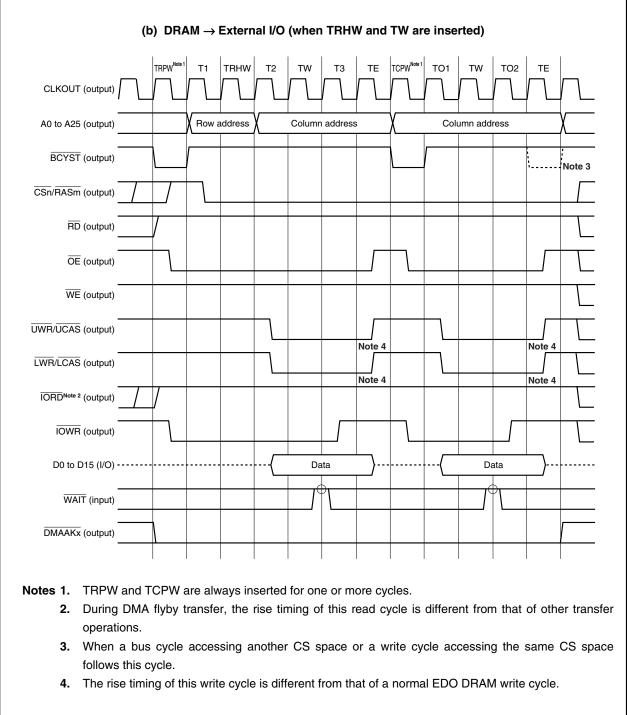
Figure 6-19. DRAM Access Timing During DMA Flyby Transfer (2/4)
