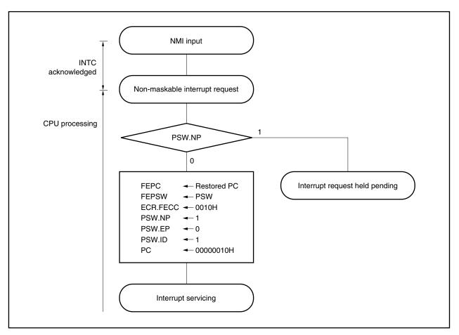
Figure 7-1. Servicing Configuration of Non-Maskable Interrupt
