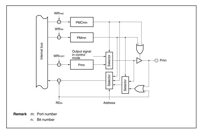
Figure 14-1. Block Diagram of Type A
