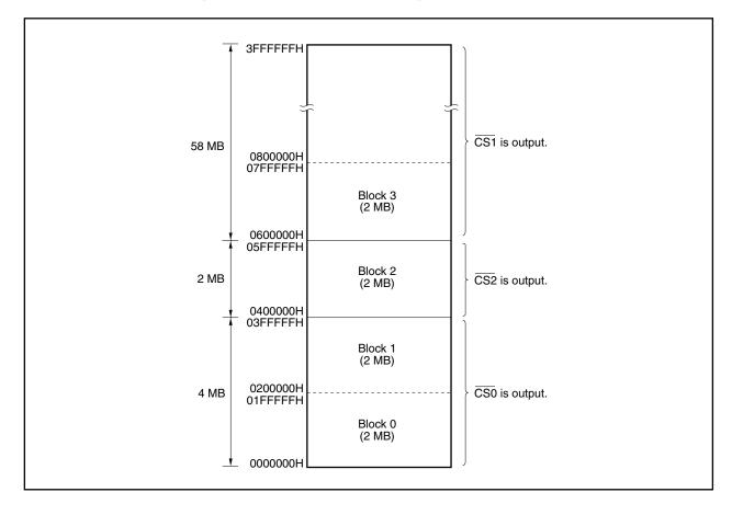
Figure 4-1. Example When CSC0 Register Is Set to 0703H
