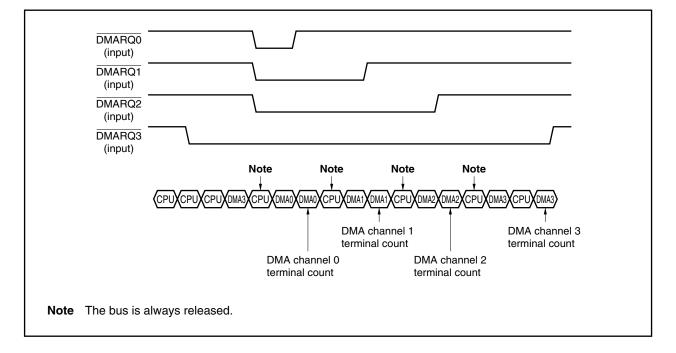
Figure 6-3. Single Transfer Example 2
