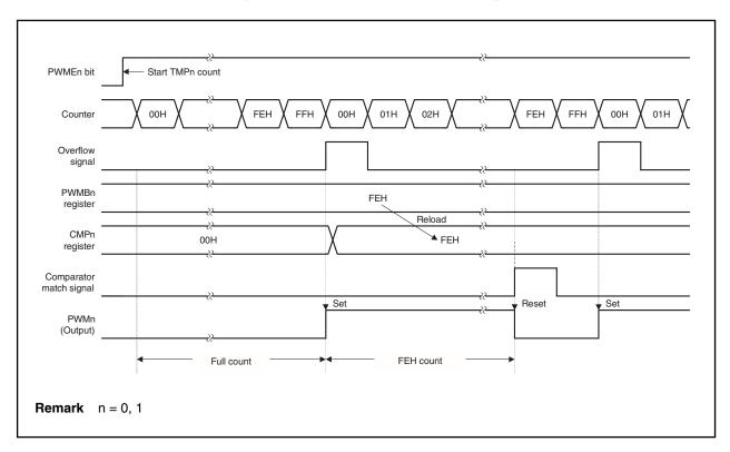
Figure 13-1. PWM Basic Operation Timing
