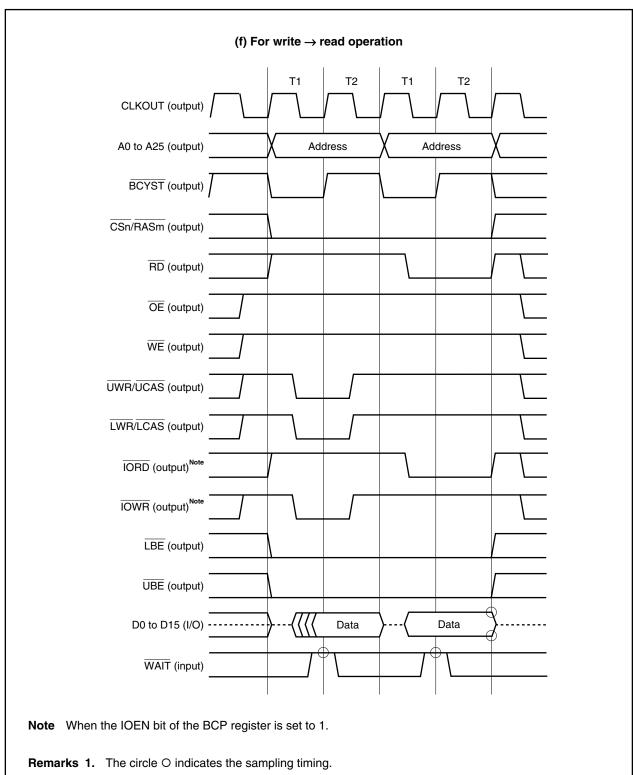
Figure 5-2. SRAM, External ROM, External I/O Access Timing (6/6)
