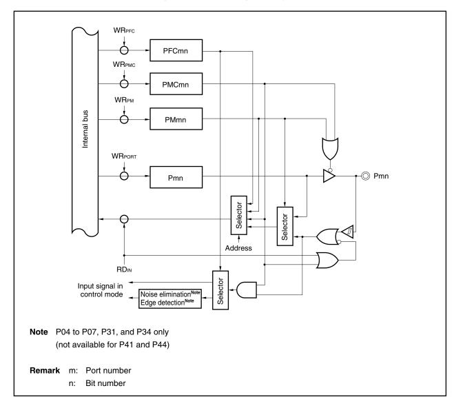
Figure 14-8. Block Diagram of Type H
