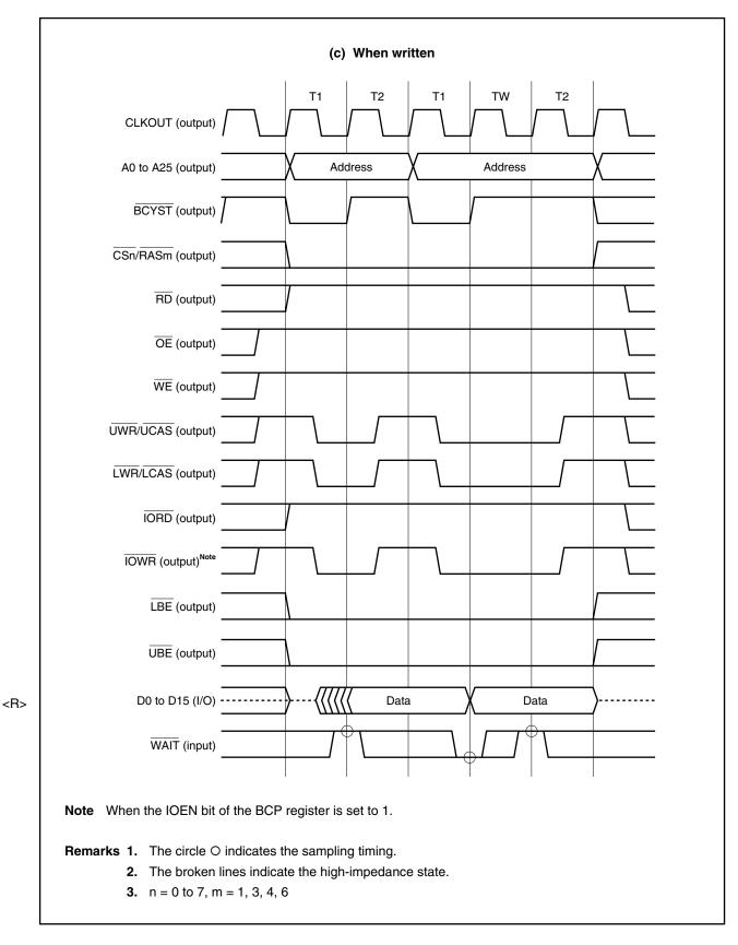
Figure 5-2. SRAM, External ROM, External I/O Access Timing (3/6)
