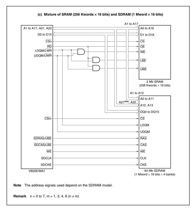
Figure 5-1. Examples of Connection to SRAM (2/2)
