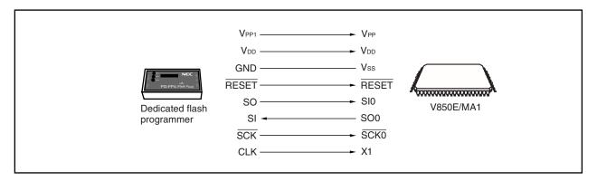
The dedicated flash programmer outputs the transfer clock and the V850E/MA1 operates as a slave.
