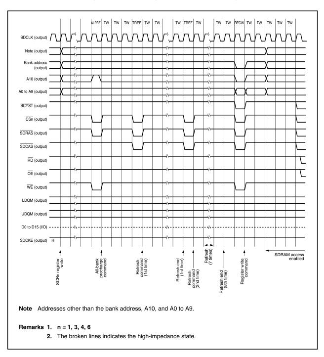
Figure 5-27. SDRAM Register Write Operation Timing
