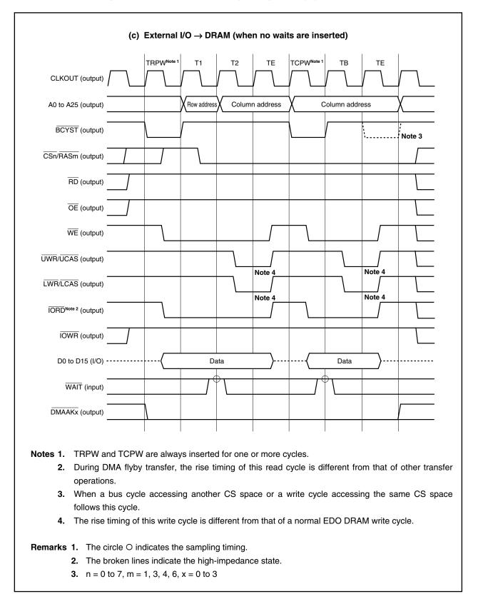
Figure 6-19. DRAM Access Timing During DMA Flyby Transfer (3/4)
