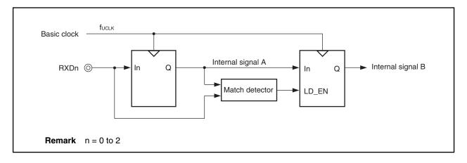
Figure 11-10. Noise Filter Circuit
