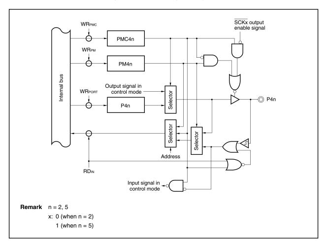
Figure 14-13. Block Diagram of Type M
