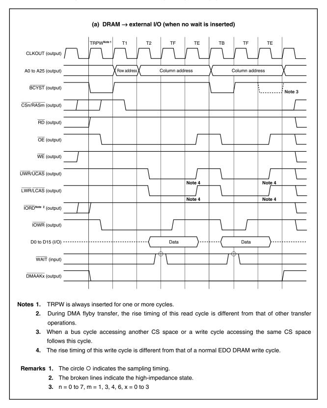
Figure 6-19. DRAM Access Timing During DMA Flyby Transfer (1/4)
