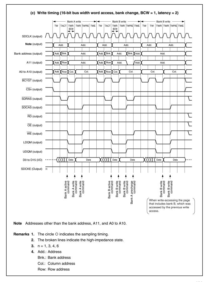
Figure 5-22. SDRAM Access Timing (3/4)
