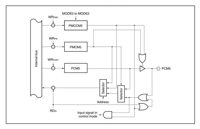
Figure 14-5. Block Diagram of Type E
