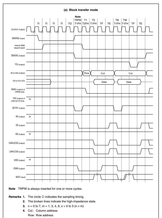
Figure 6-16. Timing of Flyby Transfer (DRAM  $\rightarrow$  External I/O) (1/3)
