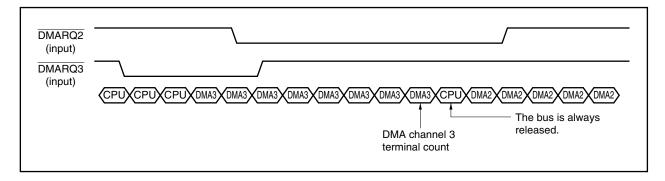
Figure 6-8. Block Transfer Example
