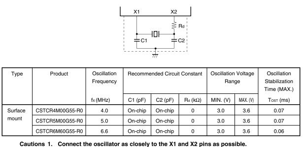
2. Do not wire any other signal lines in the area indicated by the broken lines.
