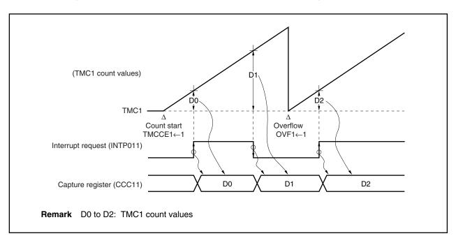
Figure 10-4. TMC1 Capture Operation Example (When Both Edges Are Specified)
