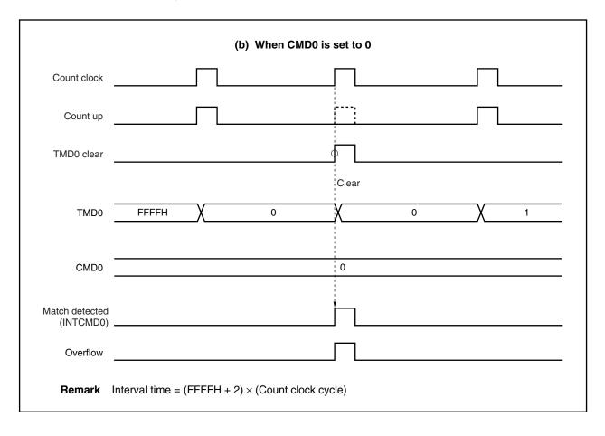
Figure 10-14. TMD0 Compare Operation Example (2/2)
