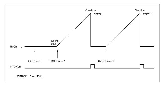
Figure 10-2. Operation After Overflow (When OSTn = 1)
