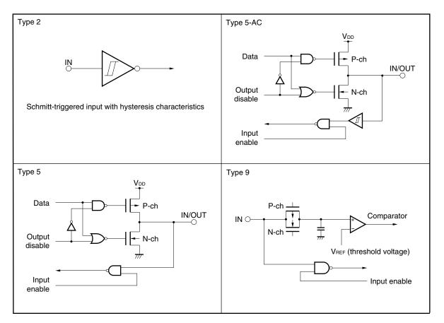
**Remark** Type 2, type 5, and type 5-AC are 5 V tolerant buffers. Design the pattern ensuring that the coupling capacitance is small.
