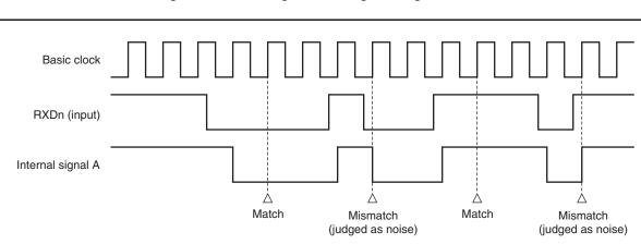
Figure 11-11. Timing of RXDn Signal Judged as Noise
