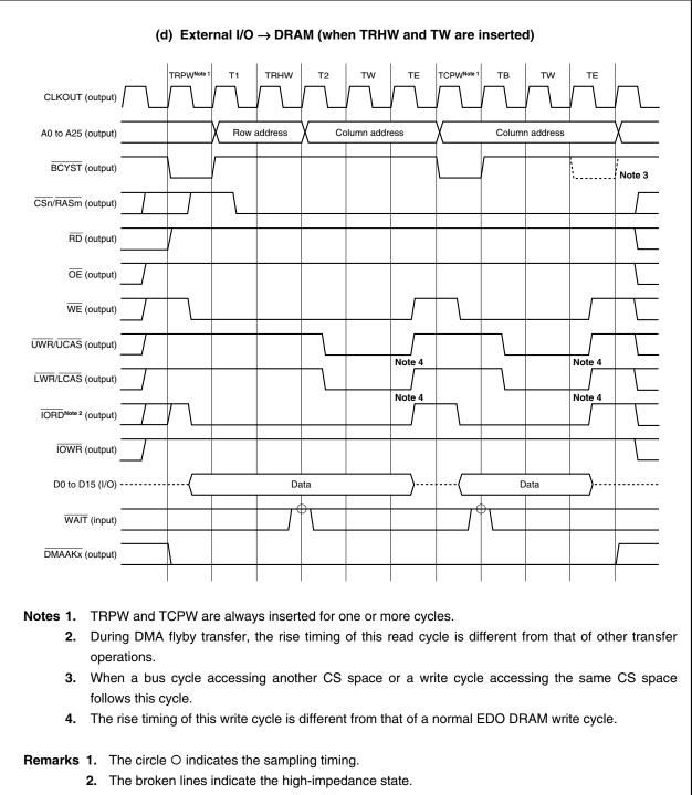
Figure 6-19. DRAM Access Timing During DMA Flyby Transfer (4/4)
