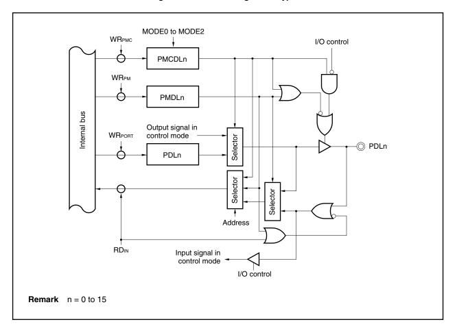
Figure 14-15. Block Diagram of Type O
