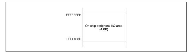
Peripheral I/O registers associated with the operating mode specification and the state monitoring for the onchip peripheral I/O are all memory-mapped to the on-chip peripheral I/O area. Program fetches cannot be executed from this area.
