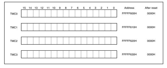
TMCn performs the count-up operations of an internal count clock or external count clock. Timer start and stop are controlled by the TMCCEn bit of timer mode control register Cn0 (TMCCn0) (n = 0 to 3).
