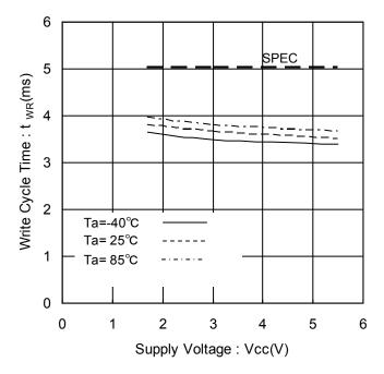
Figure 26. Write Cycle Time vs Supply Voltage
