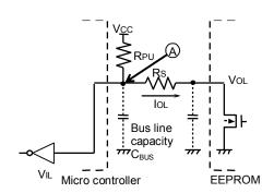
Figure 47. I/O Circuit Diagram
