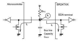
Figure 44. I/O Circuit Diagram
