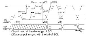
Figure 2-(a). Serial Input / Output Timing
