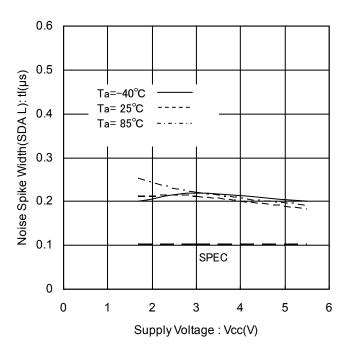
Figure 30. Noise Spike Width vs Supply Voltage  $(\operatorname{SDAL})$
