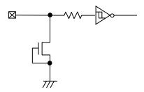
Figure 49. Input Pin Circuit Diagram
