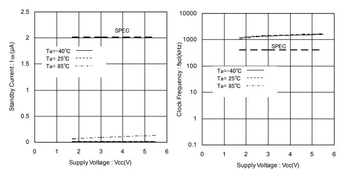
Figure 12. Standby Current vs Supply Voltage
