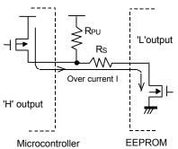
Figure 48. I/O Circuit Diagram
